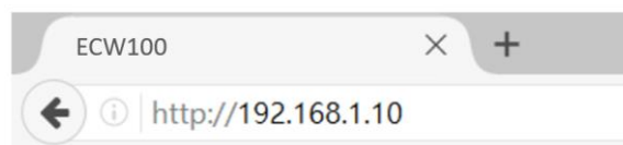
Example of entering ECW100's default IP Address via a web browser
