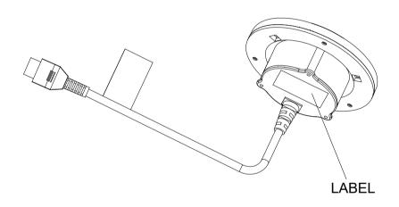
Input:5Vdc 2A,Output:5W Max Input:9Vdc 1.65A,Output:10W Max
