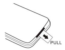
2. Remove the battery if the remote control is not used for a month or longer. If the battery is depleted remove and dispose of the old battery immediately.
