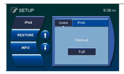
Select **Manual**, only operation via ipod is allowed Select **Full**, only operation via unit is allowed
