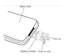
Remove the battery from the battery holder
