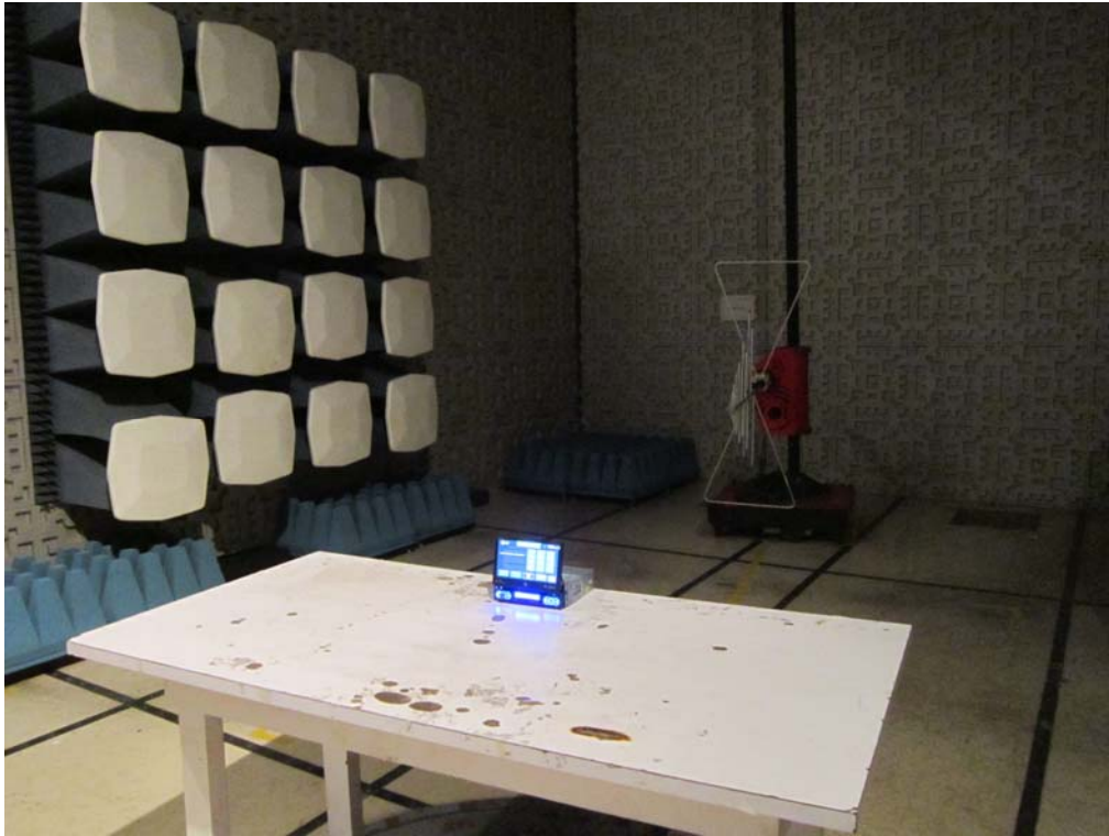
TEST SETUP OF RADIATED EMISSION (30MHz-1GHz)
