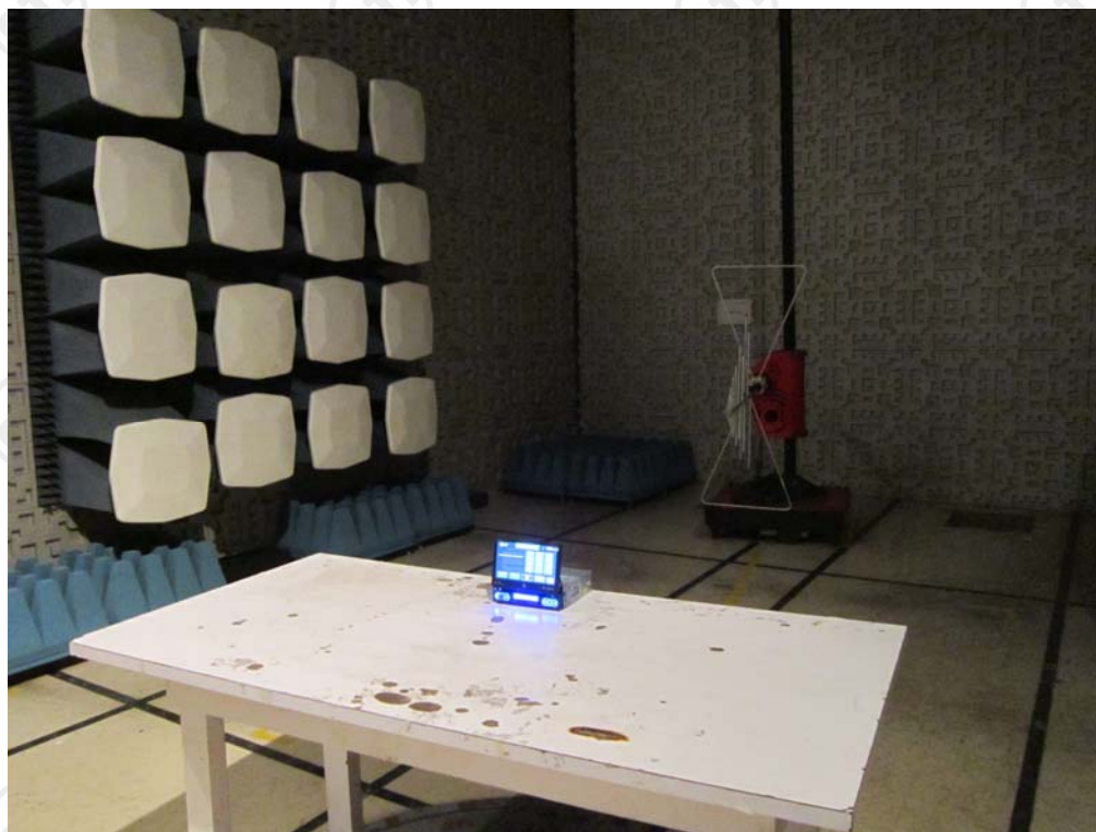
TEST SETUP OF RADIATED EMISSION (30MHz-1GHz)
