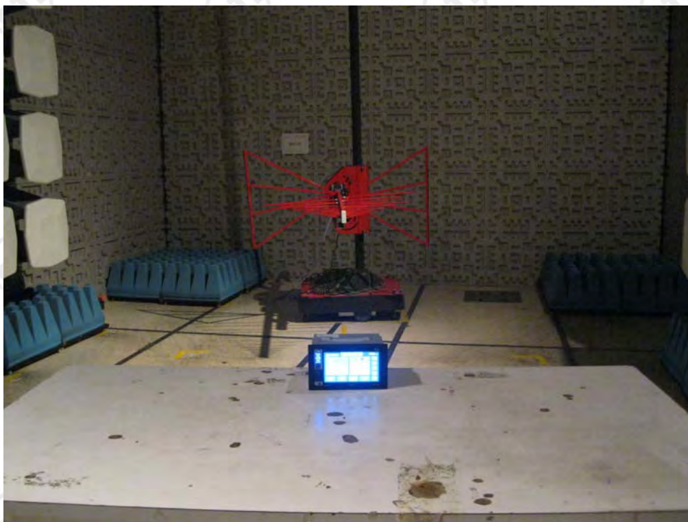
TEST SETUP OF RADIATED EMISSION (30MHz-1GHz)
