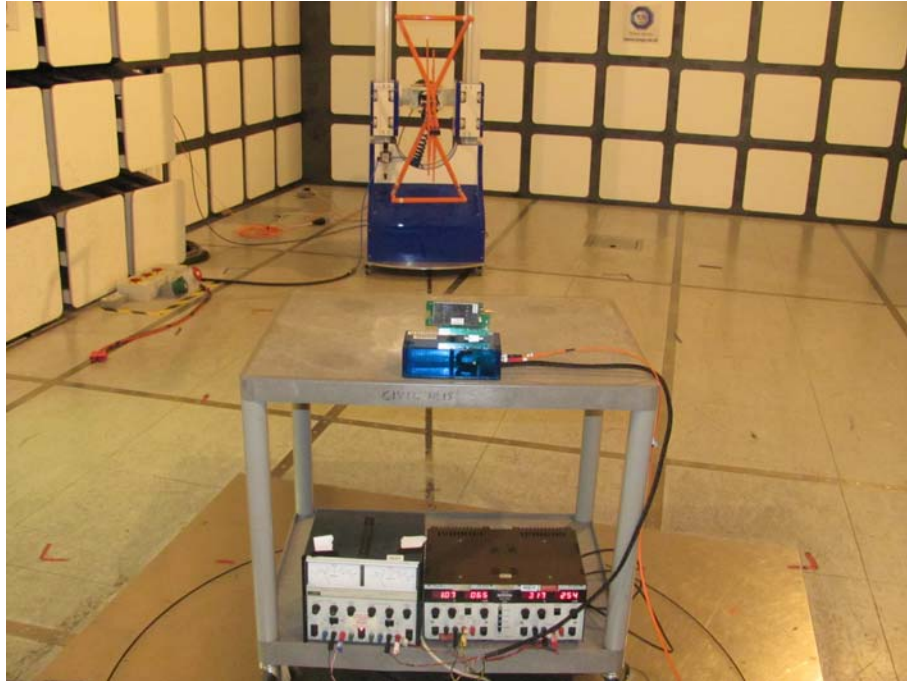
Radiated Emissions 30MHz-1GHz – PIFA Antenna
