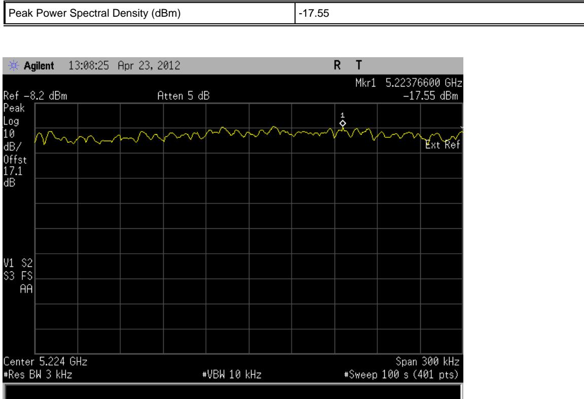
The test was performed on the worst case data rate for 802.11(n) - 40 MHz BW modulation. The worst case was deemed as the data rate which produced the highest level of conducted average power. This data rate was 135Mbps.
