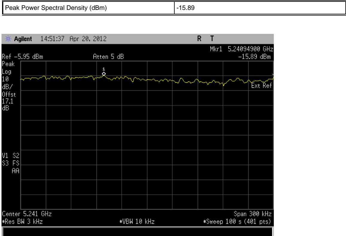
The test was performed on the worst case data rate for 802.11(n) - 20 MHz BW modulation. The worst case was deemed as the data rate which produced the highest level of conducted average power. This data rate was 21.70 Mbps.
