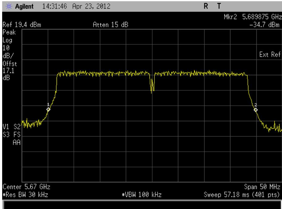
The test was performed on the worst case data rate for 802.11(n) - 40 MHz BW modulation. The worst case was deemed as the data rate which produced the highest level of conducted average power. This data rate was 135Mbps.
