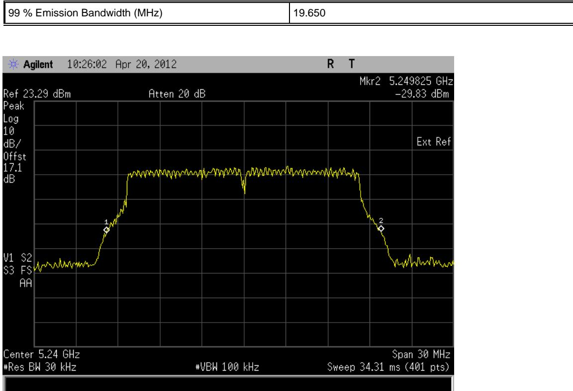
The test was performed on the worst case data rate for 802.11(a) modulation. The worst case was deemed as the data rate which produced the highest level of conducted average power. This data rate was 54Mbps.
