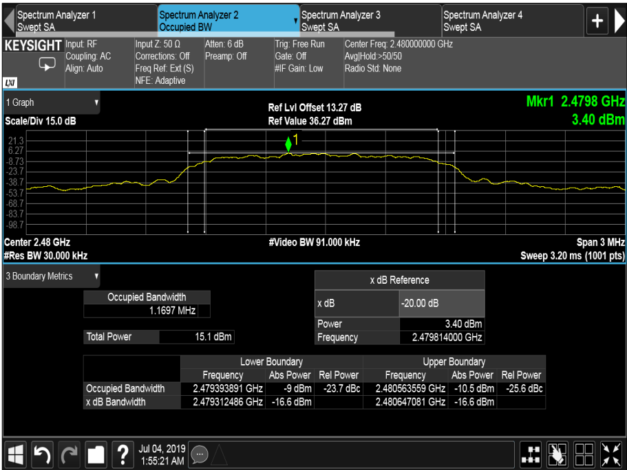
Figure 10 - 2480 MHz - \pi/4 DQPSK
