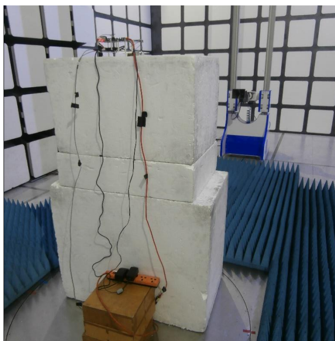
Figure 106 - Spurious Radiated Emissions - 1 GHz to 8 GHz - X Orientation
