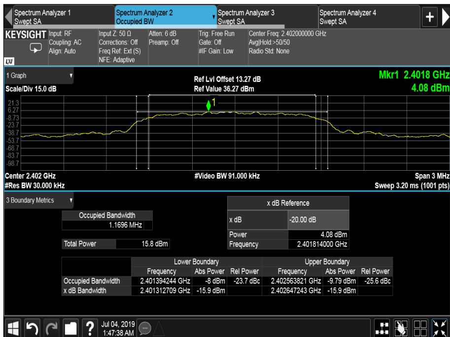
Figure 4 - 2402 MHz - \pi/4 DQPSK
