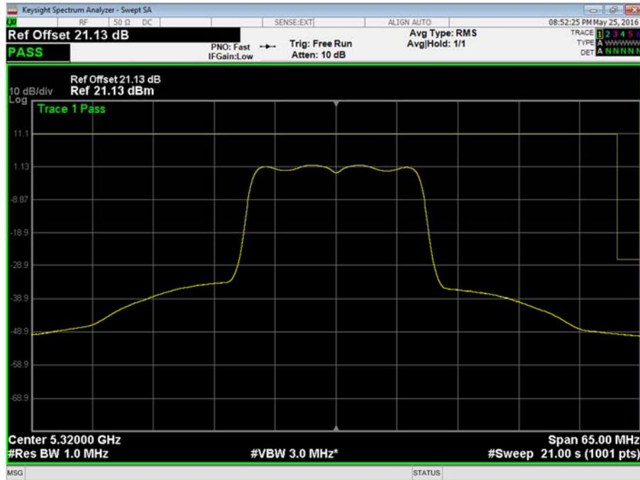
802.11n 20 MHz Bandwidth, 5320 MHz, 0°C, 5.25 V DC, Frequency Band 2, Frequency Stability Plot
