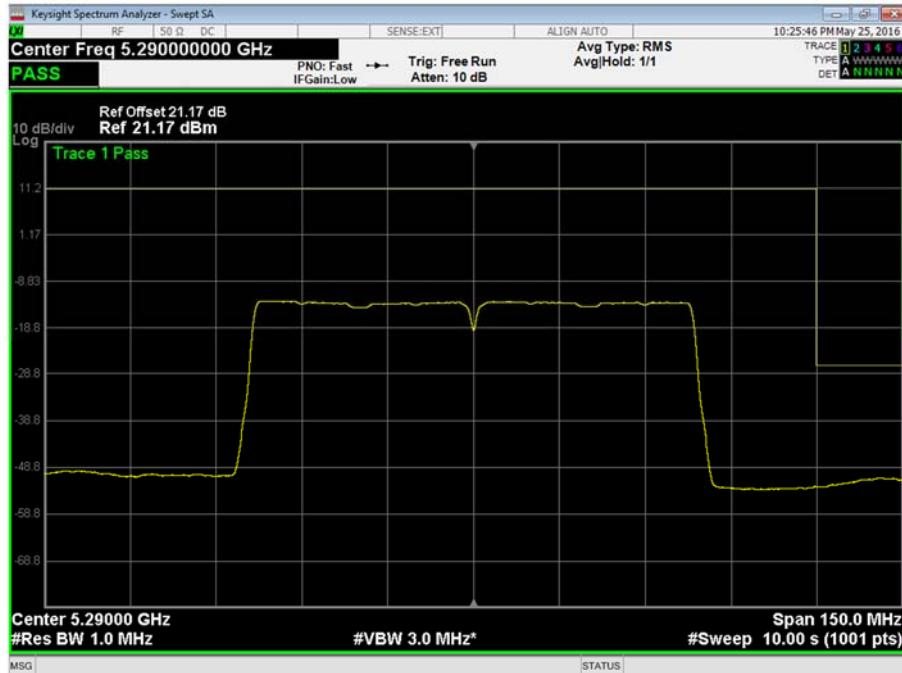
802.11ac 80 MHz Bandwidth, 5290 MHz, 0°C, 5.25 V DC, Frequency Band 2, Frequency Stability Plot
