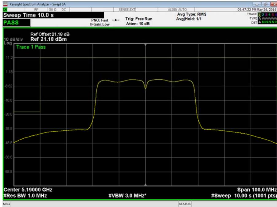
802.11n 40 MHz Bandwidth, 5190 MHz, +70°C, 5.25 V DC, Frequency Band 1, Frequency Stability Plot
