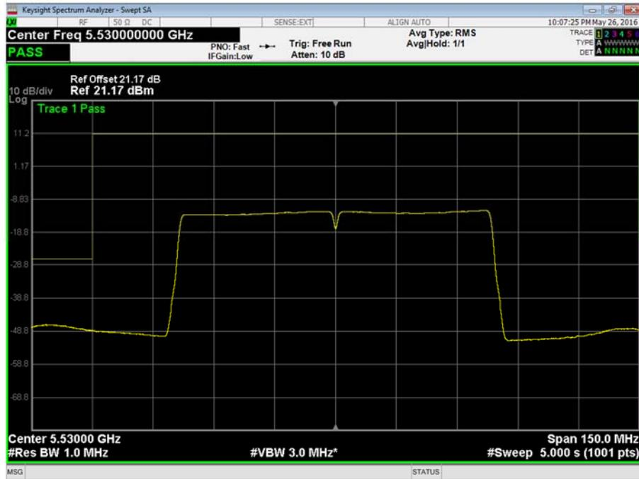
802.11ac 80 MHz Bandwidth, 5530 MHz, +70°C, 5.25 V DC, Frequency Band 3, Frequency Stability Plot
