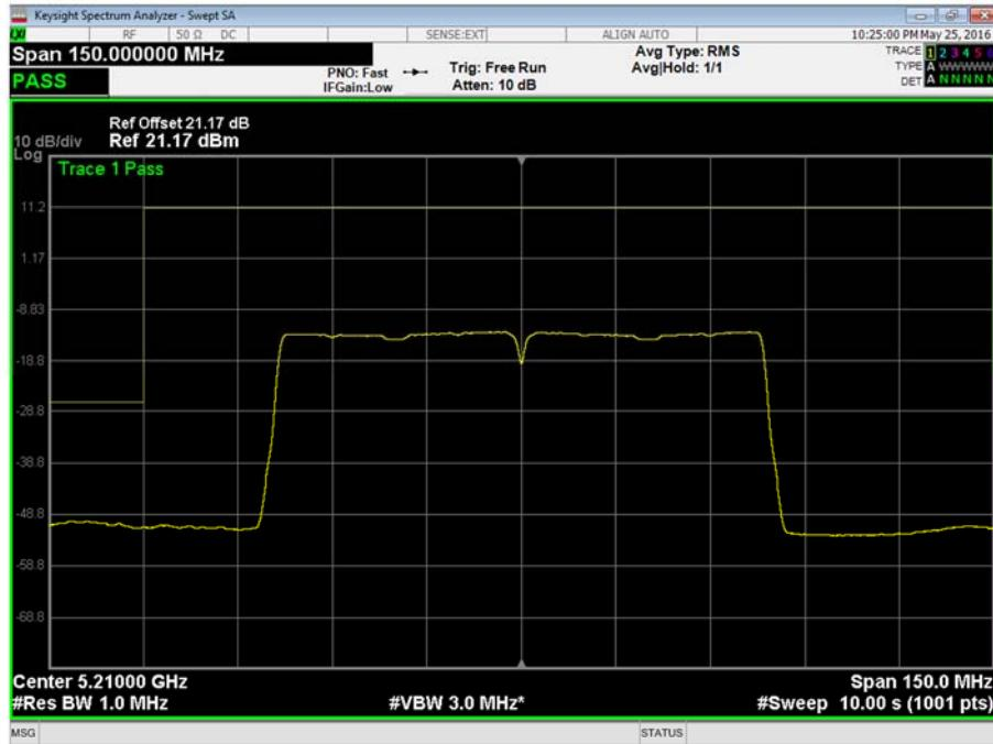
802.11ac 80 MHz Bandwidth, 5210 MHz, 0°C, 5.25 V DC, Frequency Band 1, Frequency Stability Plot
