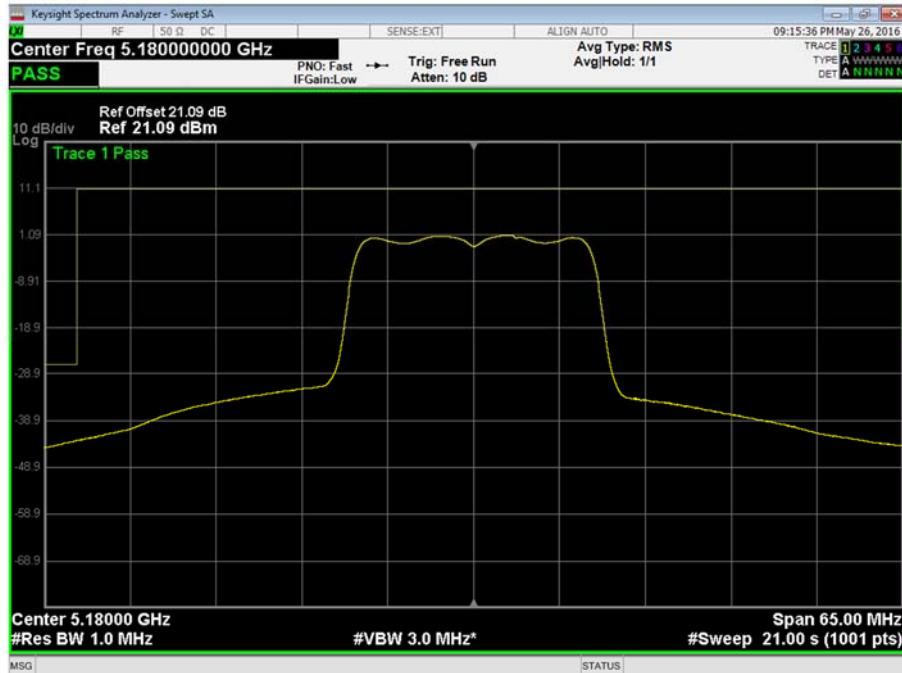
802.11n 20 MHz Bandwidth, 5180 MHz, +70°C, 5.25 V DC, Frequency Band 1, Frequency Stability Plot
