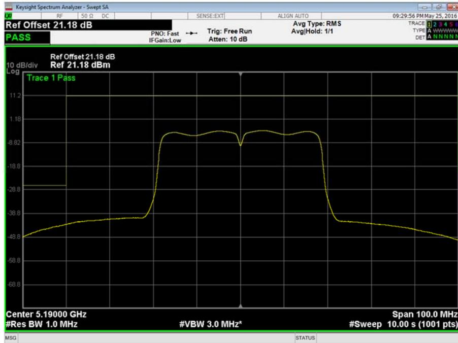
802.11n 40 MHz Bandwidth, 5190 MHz, 0°C, 5.25 V DC, Frequency Band 1, Frequency Stability Plot
