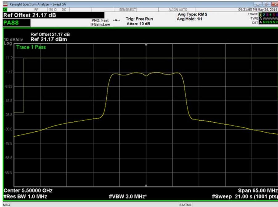
802.11n 20 MHz Bandwidth, 5500 MHz, +70°C, 5.25 V DC, Frequency Band 3, Frequency Stability Plot
