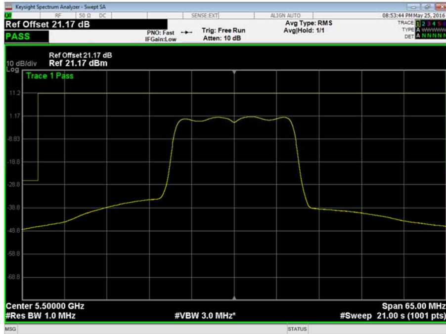
802.11n 20 MHz Bandwidth, 5500 MHz, 0°C, 5.25 V DC, Frequency Band 3, Frequency Stability Plot
