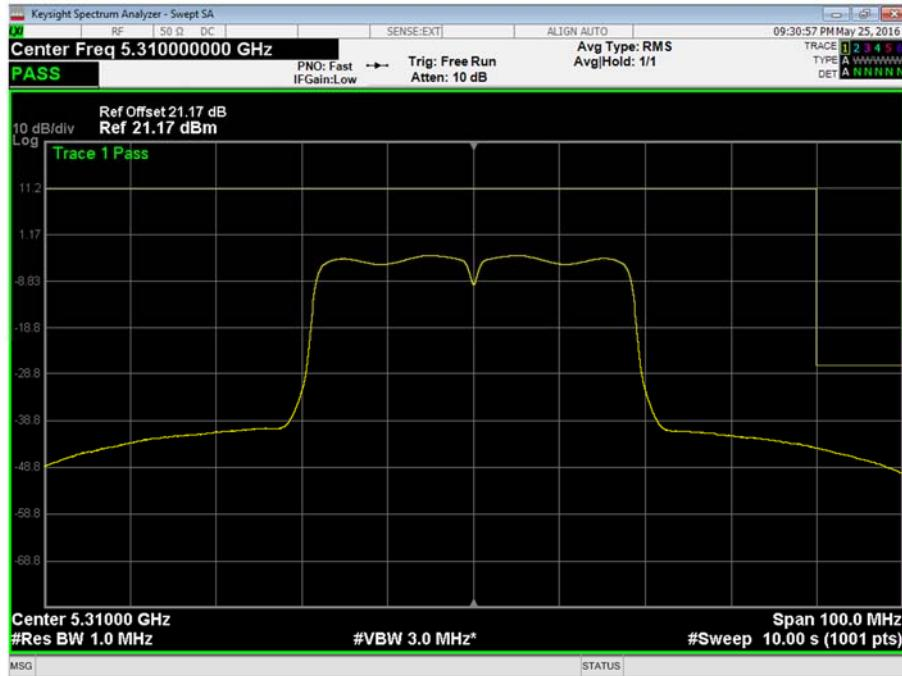
802.11n 40 MHz Bandwidth, 5310 MHz, 0°C, 5.25 V DC, Frequency Band 2, Frequency Stability Plot
