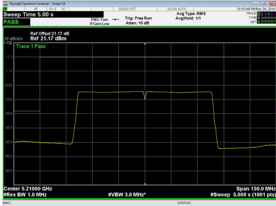
802.11ac 80 MHz Bandwidth, 5210 MHz, +70°C, 5.25 V DC, Frequency Band 1, Frequency Stability Plot
