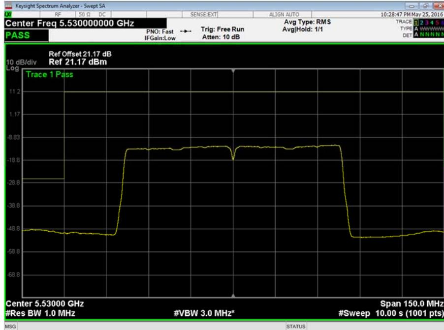
802.11ac 80 MHz Bandwidth, 5530 MHz, 0°C, 5.25 V DC, Frequency Band 3, Frequency Stability Plot
