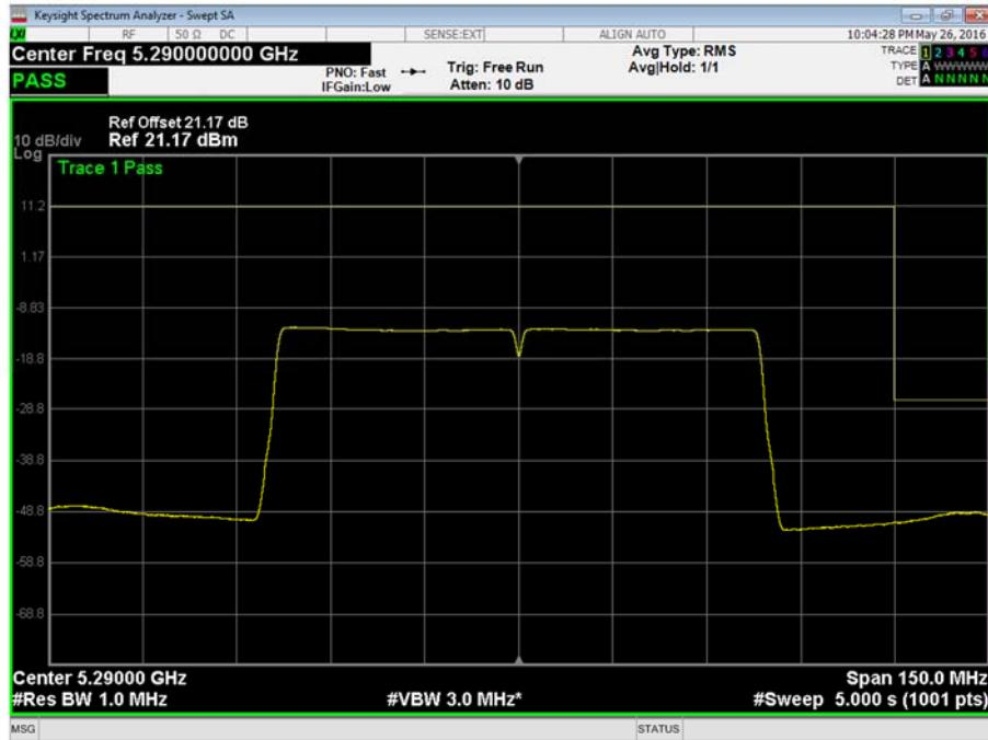
802.11ac 80 MHz Bandwidth, 5290 MHz, +70°C, 5.25 V DC, Frequency Band 2, Frequency Stability Plot
