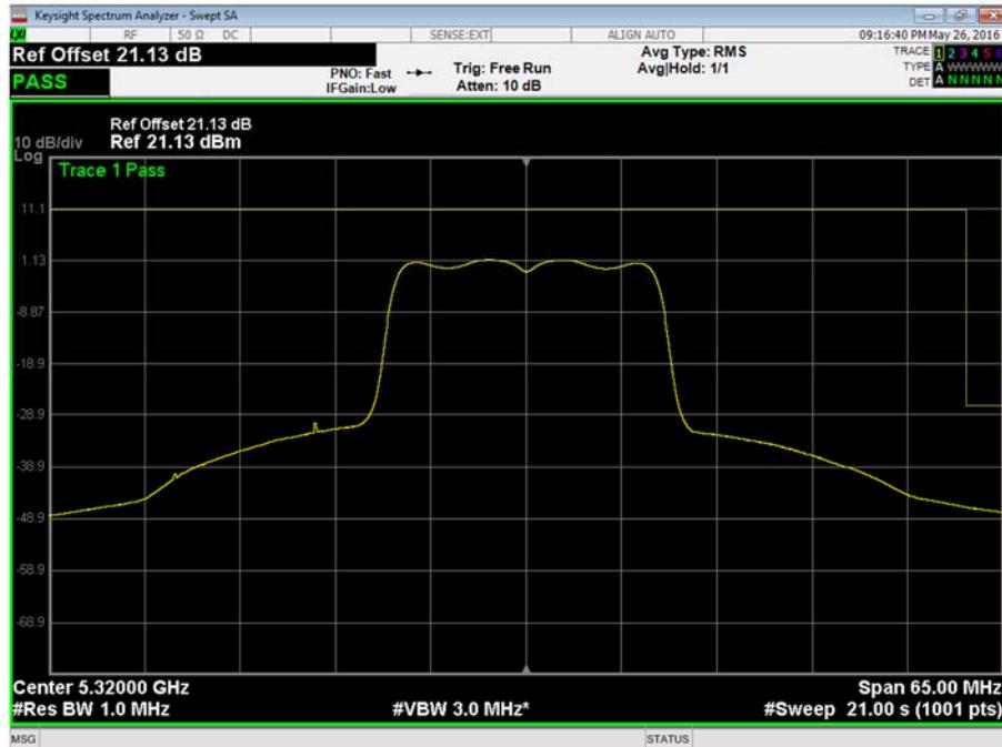
802.11n 20 MHz Bandwidth, 5320 MHz, +70°C, 5.25 V DC, Frequency Band 2, Frequency Stability Plot
