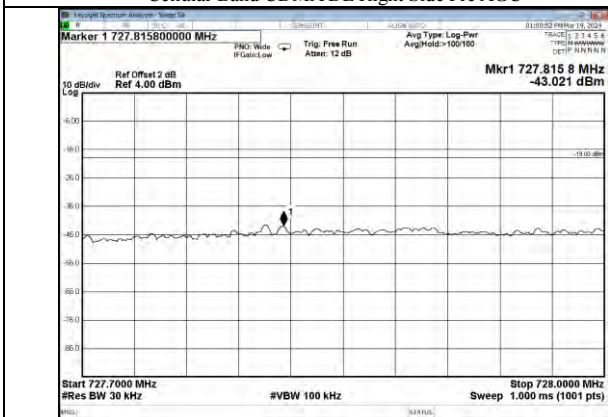
Lower 700MHz band CDMA DL Left Side Pre AGC
