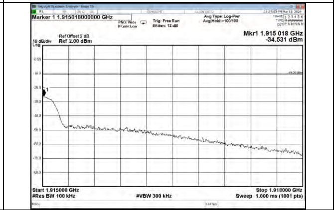
PCS Band LTE UL Right Side 10dB Above AGC
