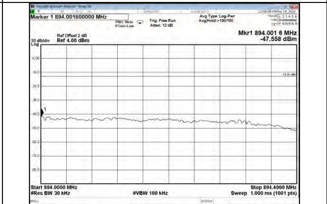
Cellular Band CDMA DL Right Side 10dB Above AGC
