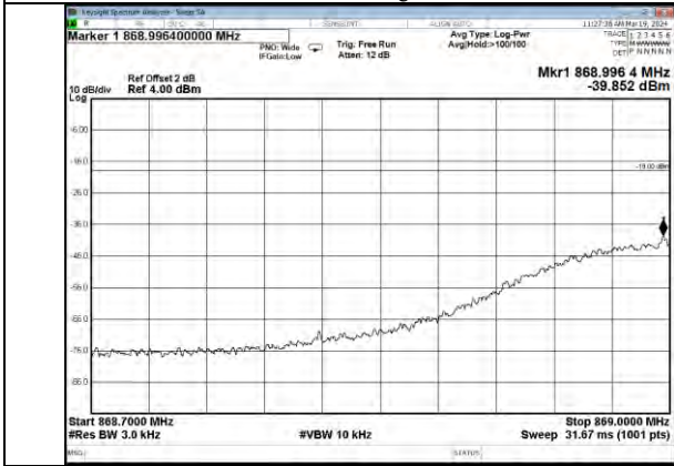
Cellular Band GSM DL Left Side Pre AGC
