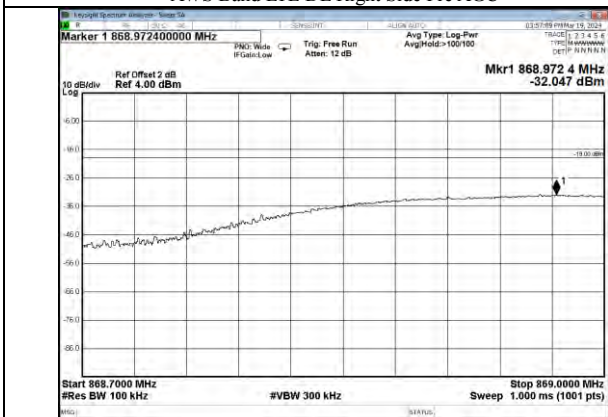
Cellular Band LTE DL Left Side Pre AGC
