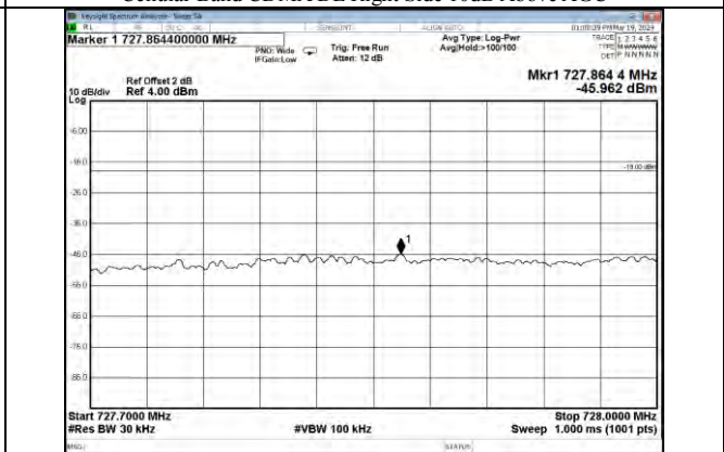
Lower 700MHz band CDMA DL Left Side 10dB Above AGC
