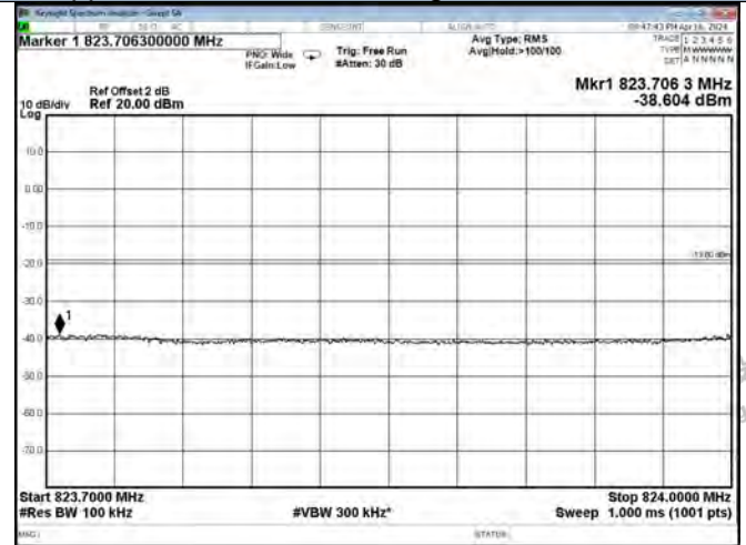
Cellular Band UL-LTE Left Side AGC+10dB
