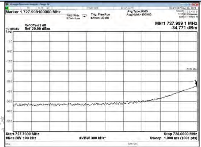
Lower 700 Band DL-GSM Left Side AGC+10dB
