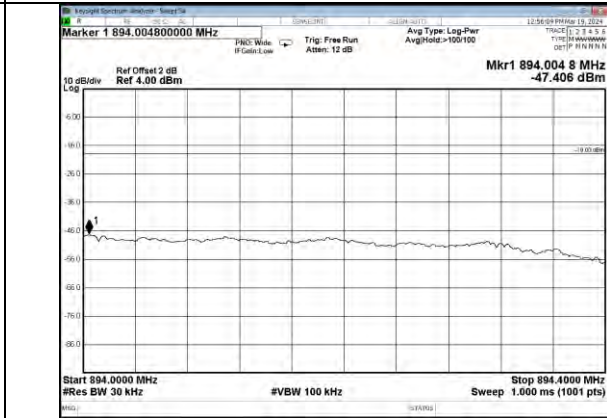
Cellular Band CDMA DL Right Side 10dB Above AGC
