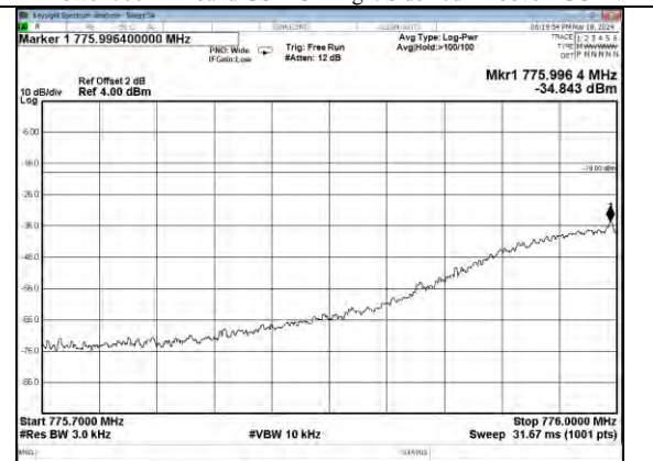
Upper 700MHz band UL Left Side 10dB Above AGC
