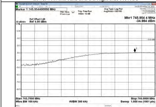
Upper 700MHz band LTE DL Left Side Pre AGC
