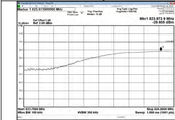
Cellular Band LTE UL Left Side Pre AGC
