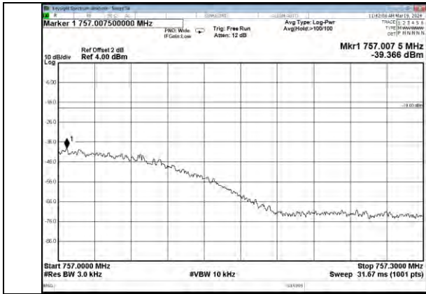
Upper 700MHz band GSM DL Right Side Pre AGC
