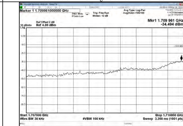
AWS Band CDMA UL Left Side 10dB Above AGC
