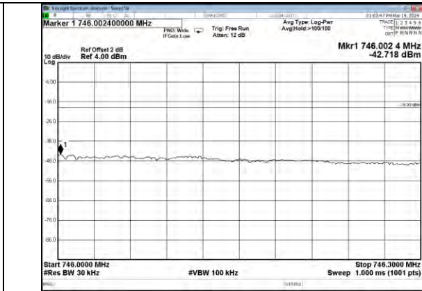
Lower 700MHz band CDMA DL Right Side 10dB Above AGC
