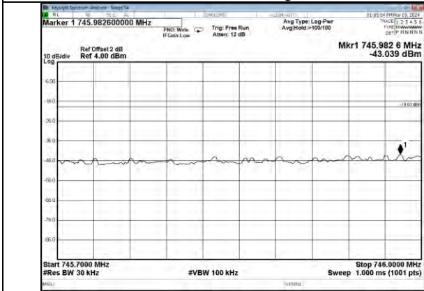
Upper 700MHz band CDMA DL Left Side Pre AGC
