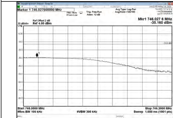
Lower 700MHz band LTE DL Right Side Pre AGC
