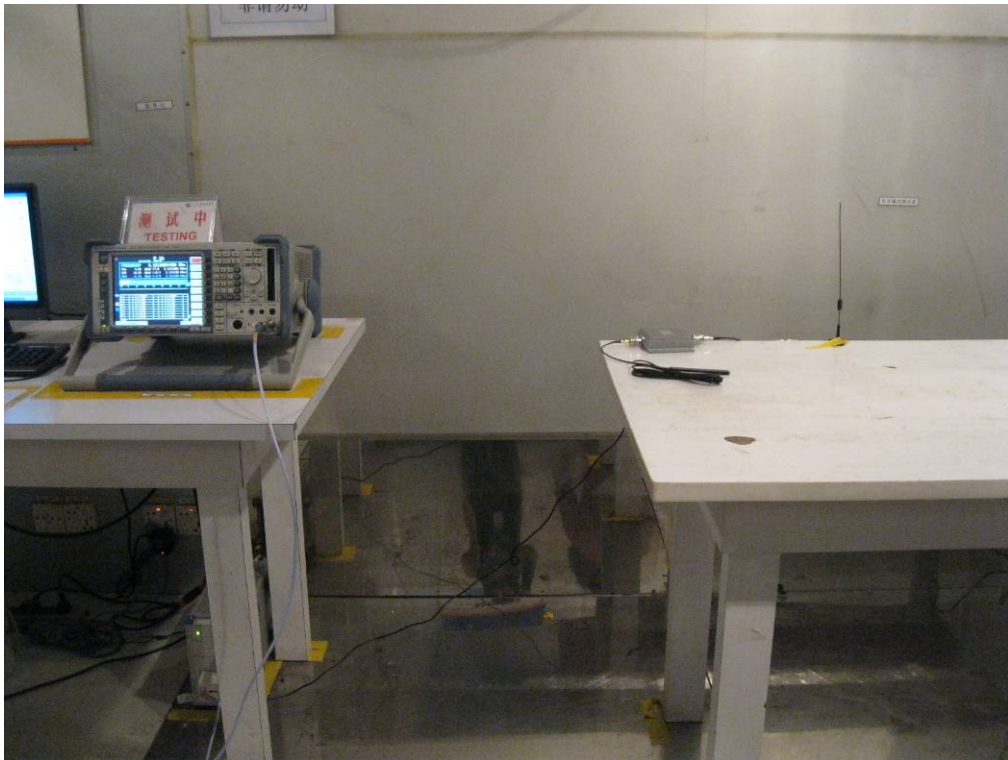
TEST SETUP OF CONDUCTED EMISSION
