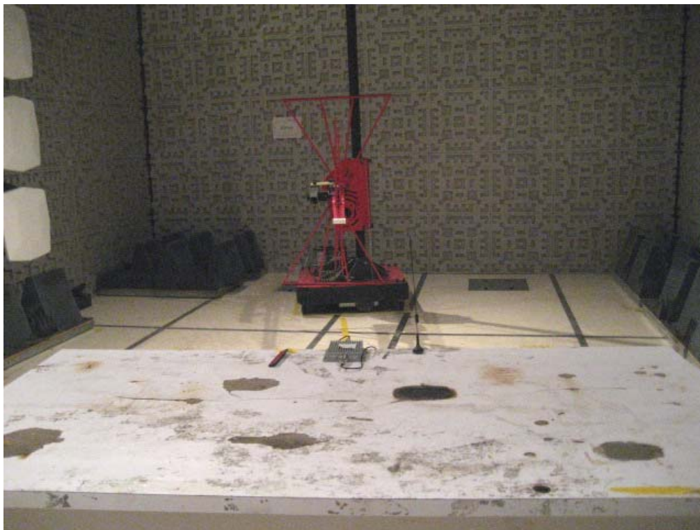
TEST SETUP OF RADIATED EMISSION
