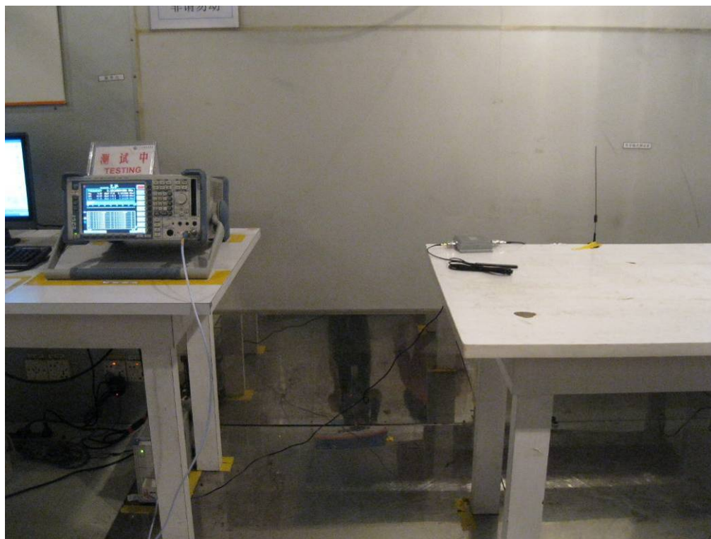
TEST SETUP OF CONDUCTED EMISSION
