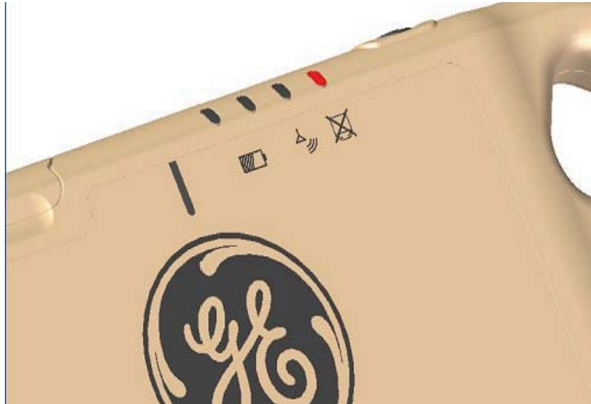
Figure 13-15 Detector fault condition
