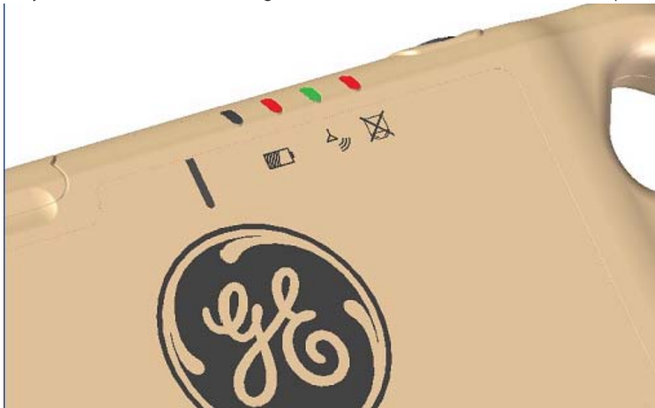
Figure 13-12 Battery less than 10% remaining; Wireless link connected; Detector exposure not allowed
