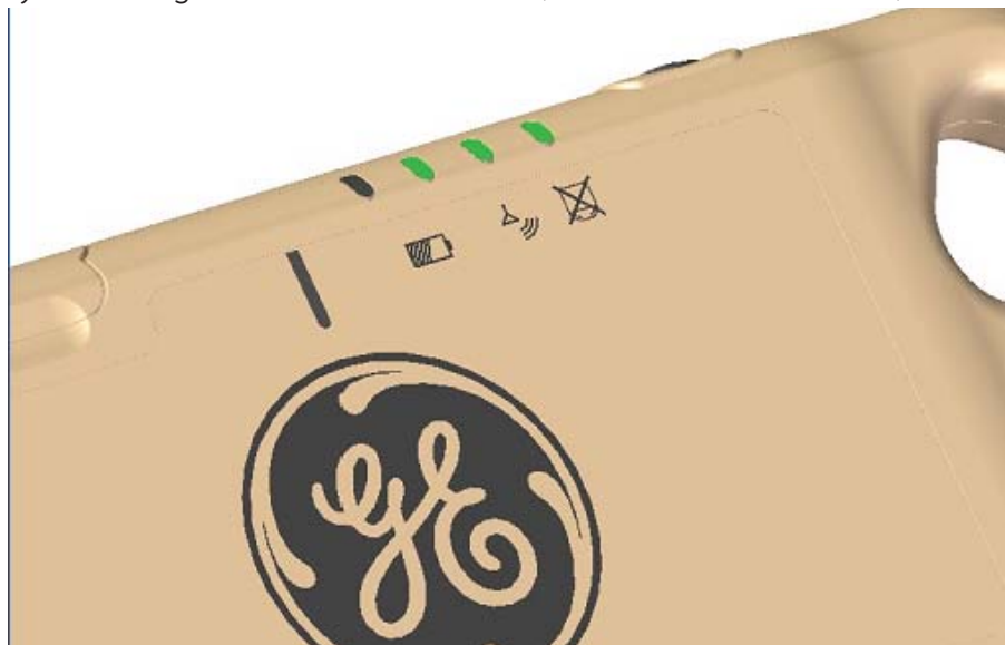
Figure 13-10 Battery remaining between 25% and 75% ; Wireless link connected; Detector ready
