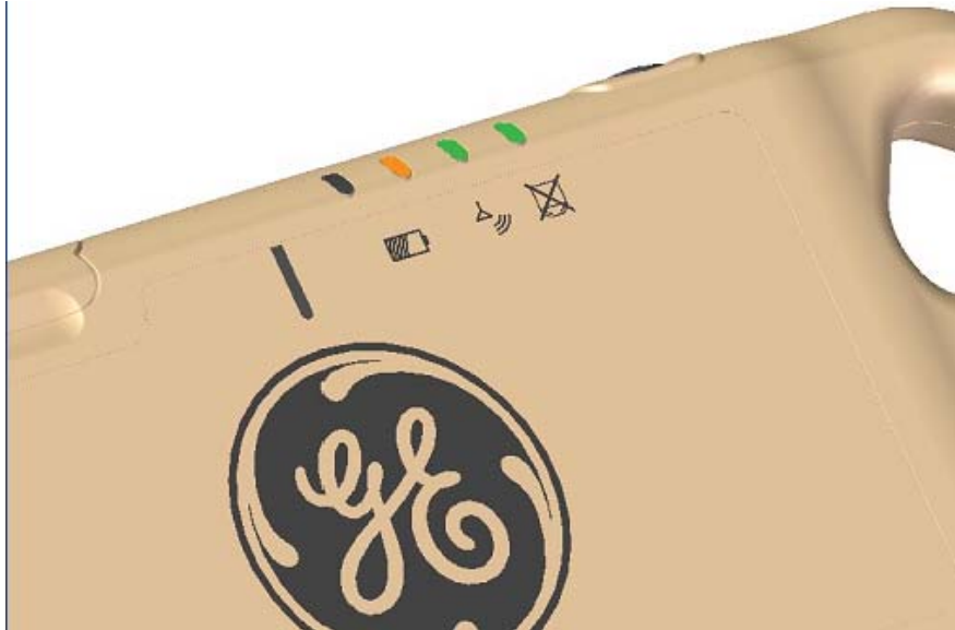
Figure 13-11 Battery remaining between 10% and 25% ; Wireless link connected; Detector ready
