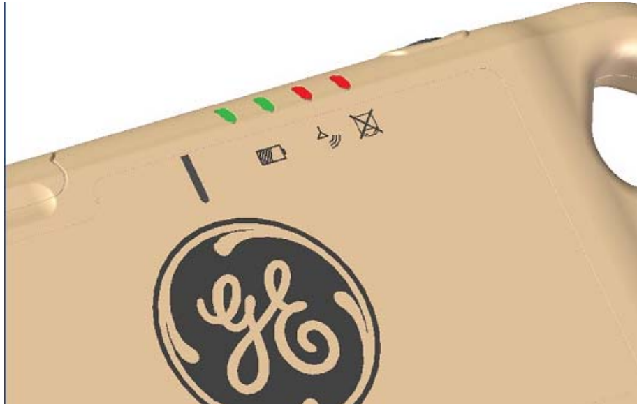
Figure 13-13 Battery more than 50% remaining; No Wireless link; Detector exposure not allowed
