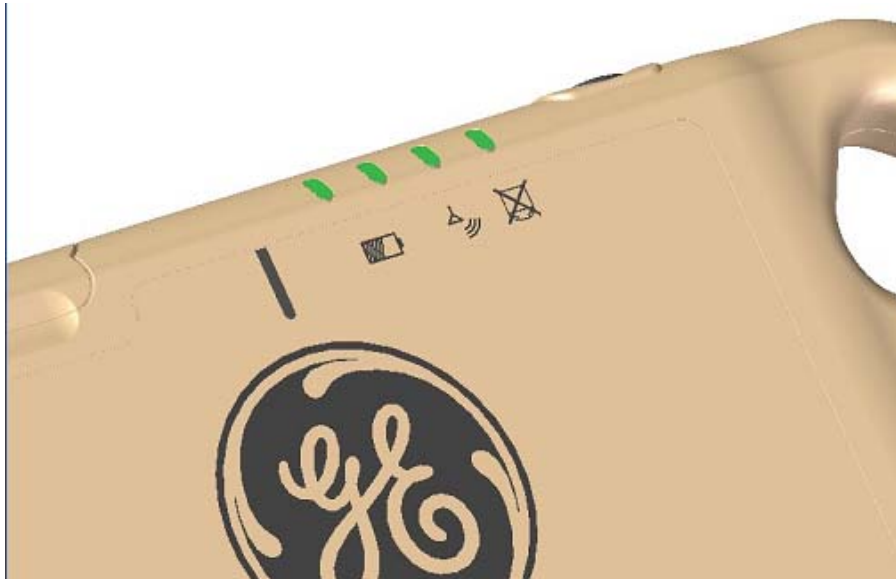
Figure 13-9 Battery more than 75% remaining; Wireless link connected; Detector ready
