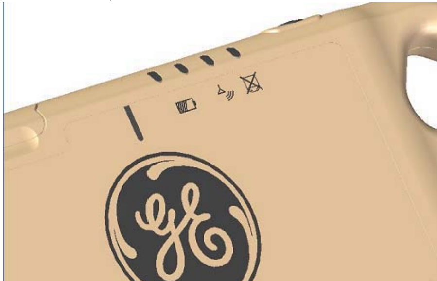
Figure 13-14 Detector off (in sleep mode)
