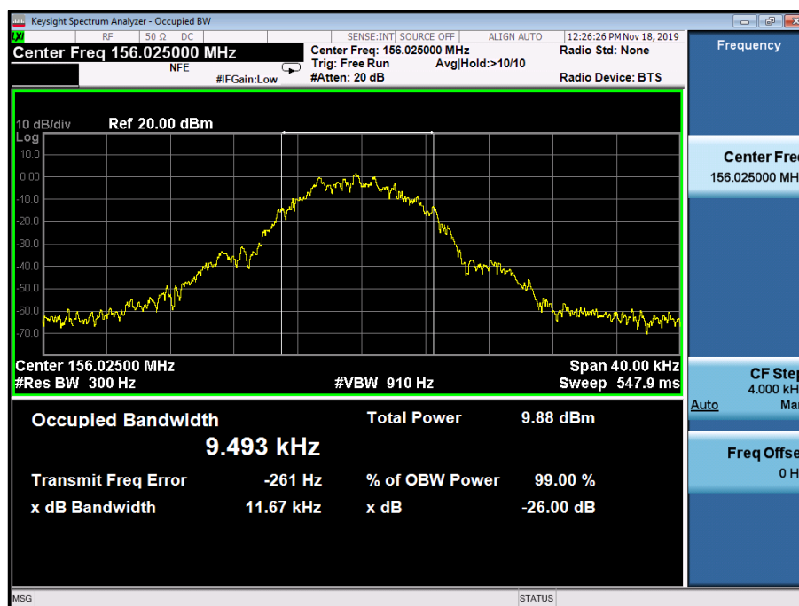
Figure 3 - 156.025 MHz Occupied Bandwidth
