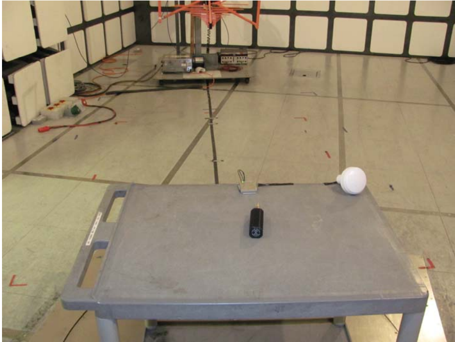
Radiated Emissions (Enclosure Port)
