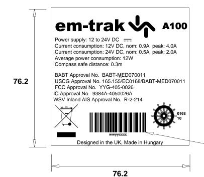
BARCODE TYPE CODE128 DETAILING 8 DIGIT UNIT SERIAL NUMBER
