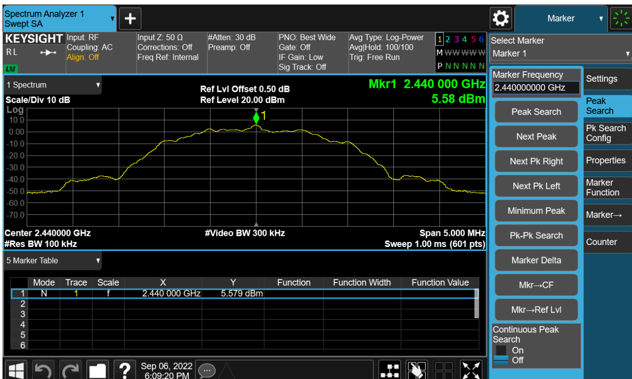
Figure 40: The plots of Conducted Spurious Emission & Authorized-band band-edge, 2440MHz, BLE-2M, Carrier Level
