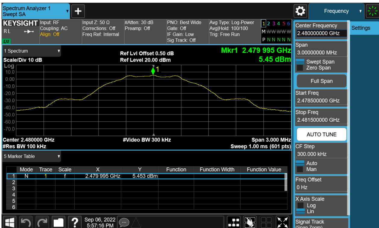
Figure 4: The plots of Conducted Spurious Emission & Authorized-band band-edge, 2480MHz, BLE-1M, Carrier Level
