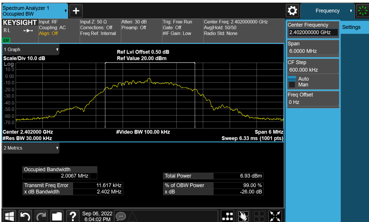
Figure 14: The plots of 99% Bandwidth, BLE-2M, 2402MHz
