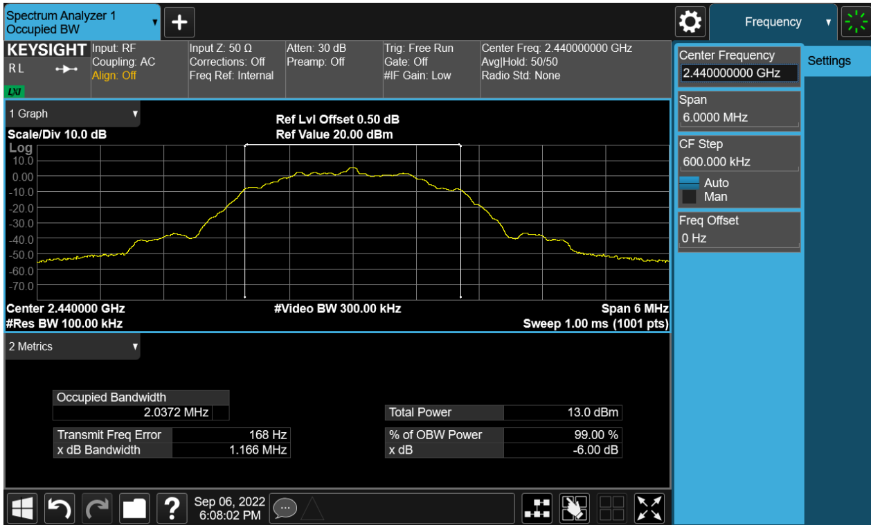
Figure 16: The plots of 99% Bandwidth, BLE-2M, 2440MHz
