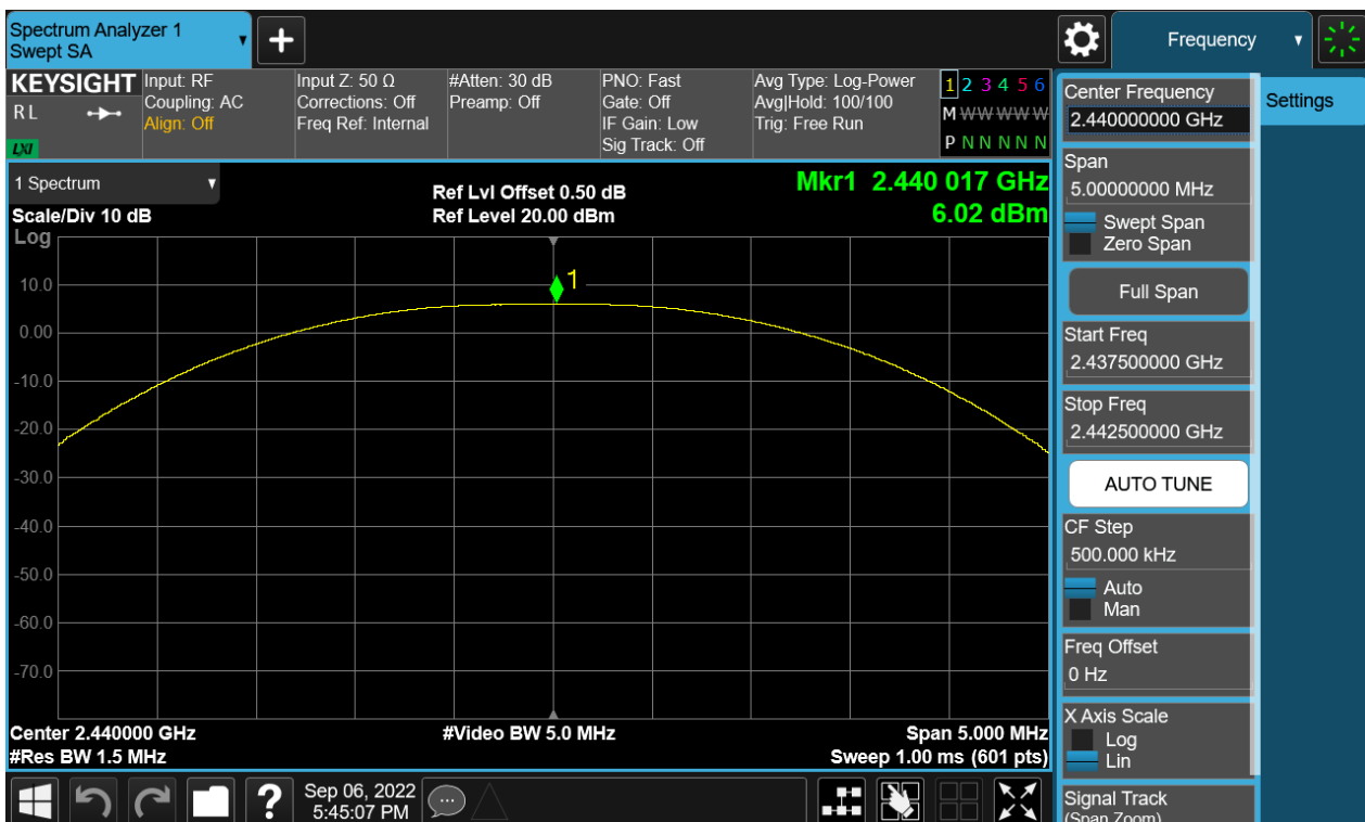
Figure 2: The plots of Peak Conducted Output Power, BLE-1M, 2440MHz
