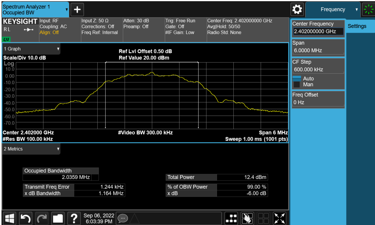
Figure 14: The plots of 99% Bandwidth, BLE-2M, 2402MHz
