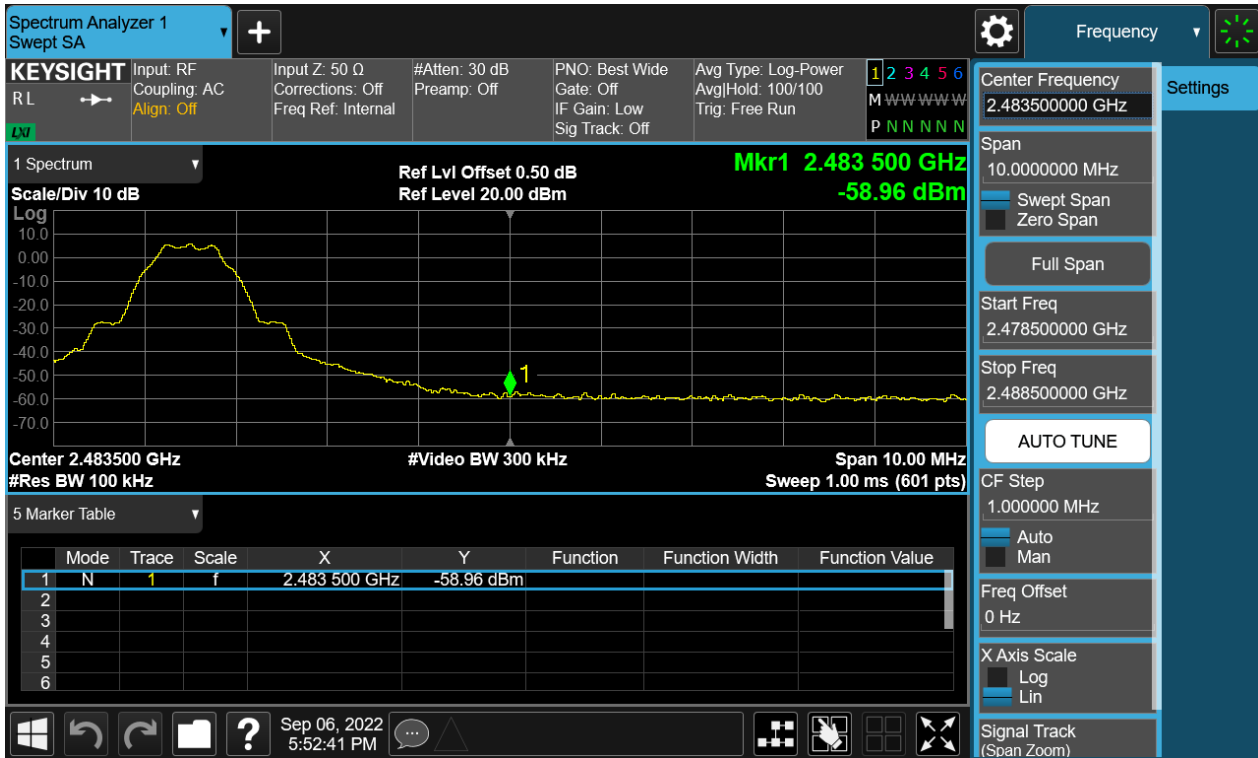
Figure 6: The plots of Conducted Spurious Emission & Authorized-band band-edge, 2480MHz, BLE-1M, Conducted spurious emissions 30MHz-3GHz
