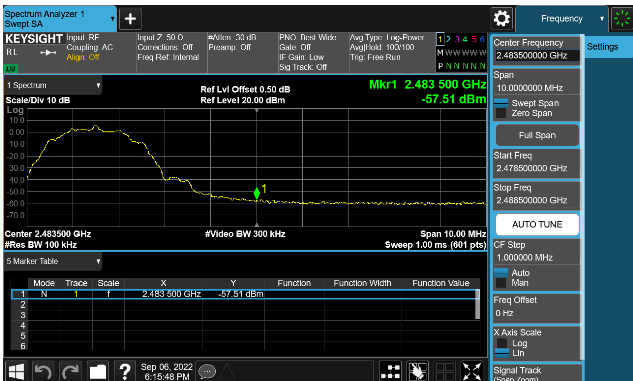
Figure 9: The plots of Conducted Spurious Emission & Authorized-band band-edge, 2480MHz, BLE-2M, Band Edge
