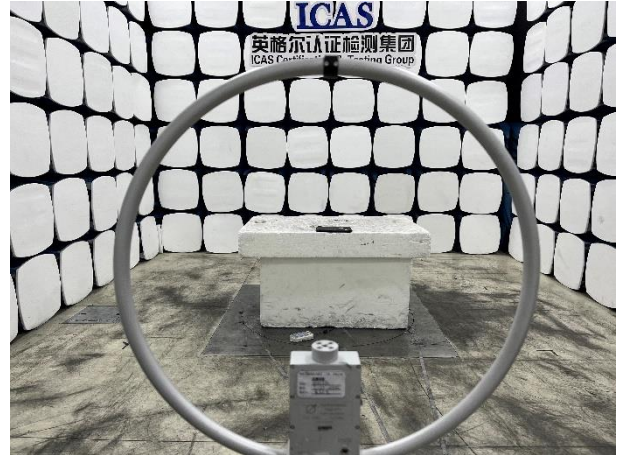
Radiated Emission Test Set-up for Below 30MHz
