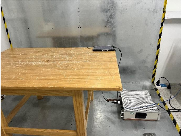
Radiated Emission Test Set-up for 30M-1GHz
