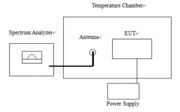
The EUT which is powered by the Battery, is coupled to the Spectrum Analyzer; the RF load attached to the EUT antenna terminal is 500hm; the path loss as the factor is calibrated to correct the reading
