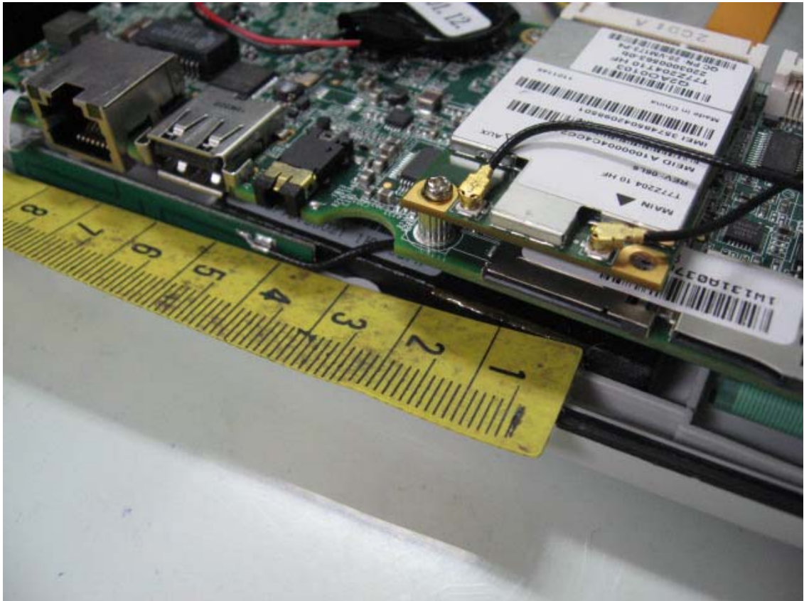
2G/3G Mobile Transmit Antenna Location
