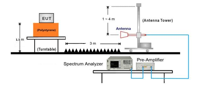
18GHz ~25GHz Test Setup:
