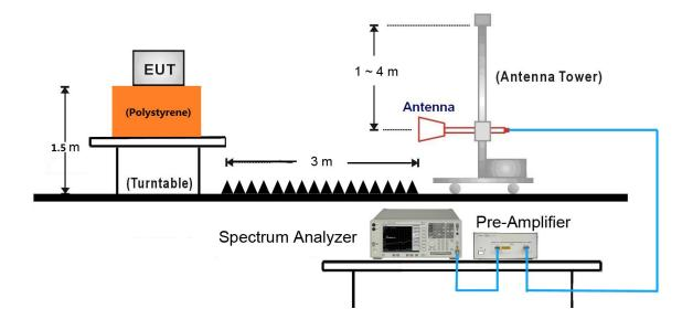
18GHz ~40GHz Test Setup:
