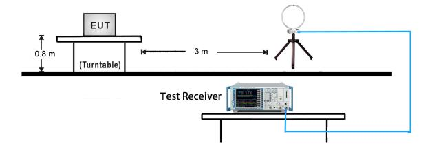
30MHz ~ 1GHz Test Setup:
