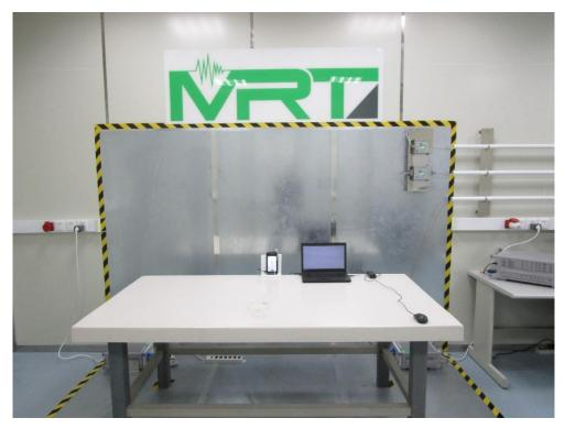
Test Mode 1~4 Description: Back View of Conducted Emission Test Setup
