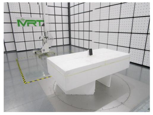
Test Mode: Mode 1~4 Description: Radiated Emission Test Setup for Above 1GHz
