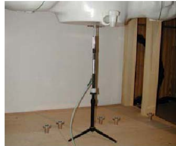
Figure 11.1 Dipole Verification Test Setup Diagram & Photo
