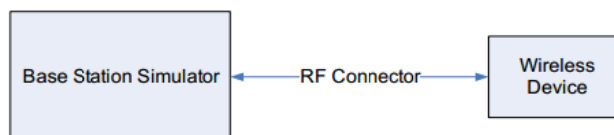
Figure 10.1 Power Measurement Setup
