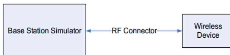
Figure 10.1 Power Measurement Setup
