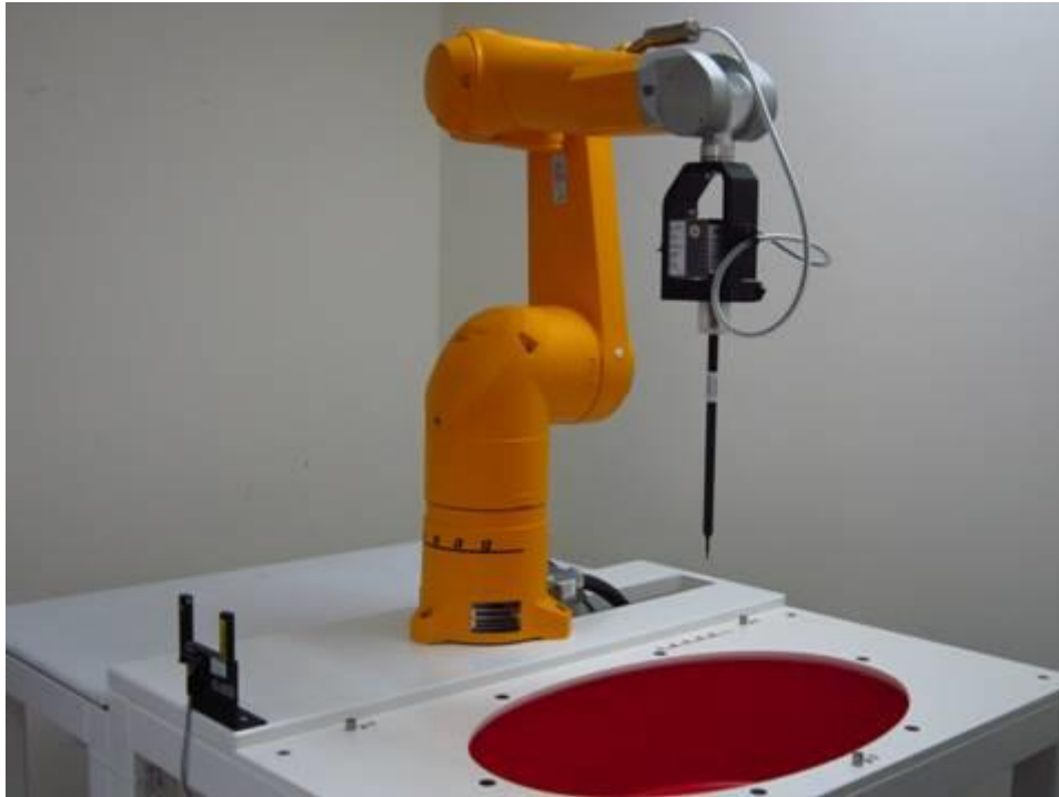
Fig.1 Photograph of the SAR measurement system
