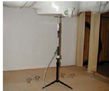
Figure 11.1 Dipole Verification Test Setup Diagram & Photo
