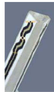
Figure 3.3 Probe Thick-Film Technique
