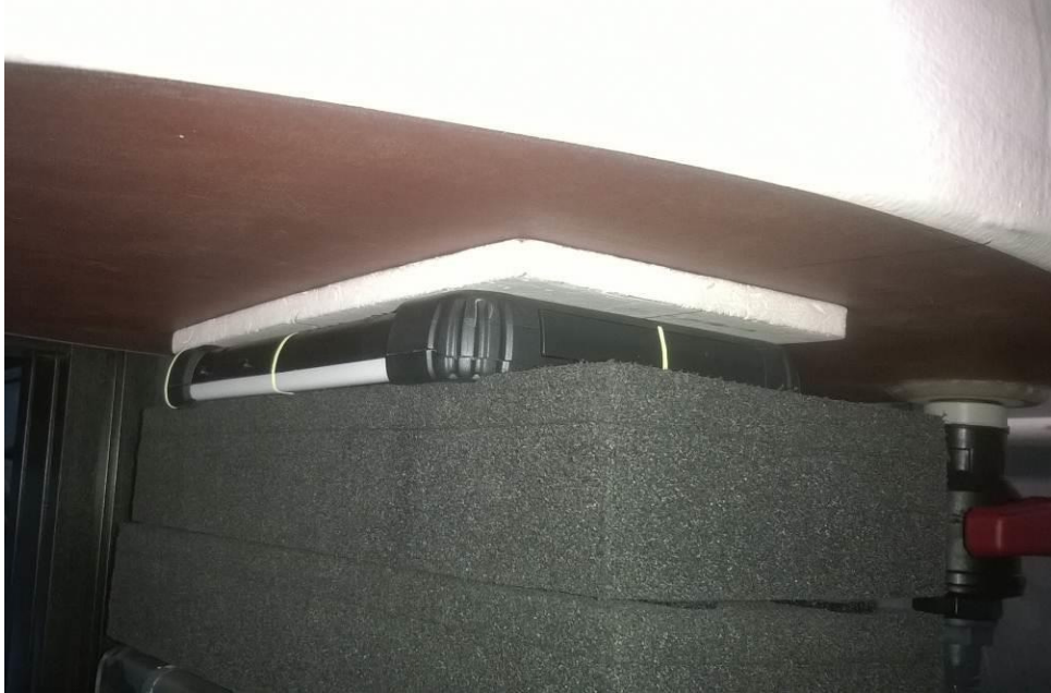
SAR Test Setup_10mm Spacer
