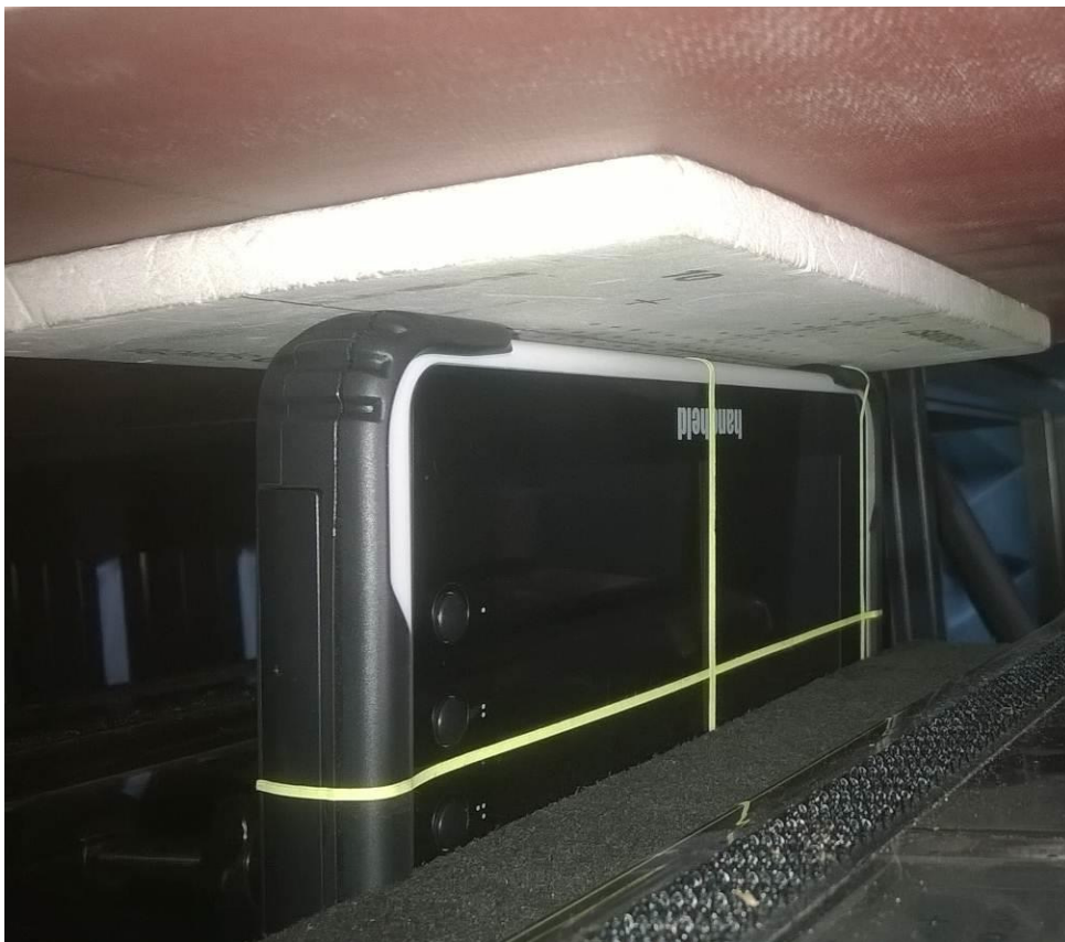
SAR Test Setup_10mm Spacer
