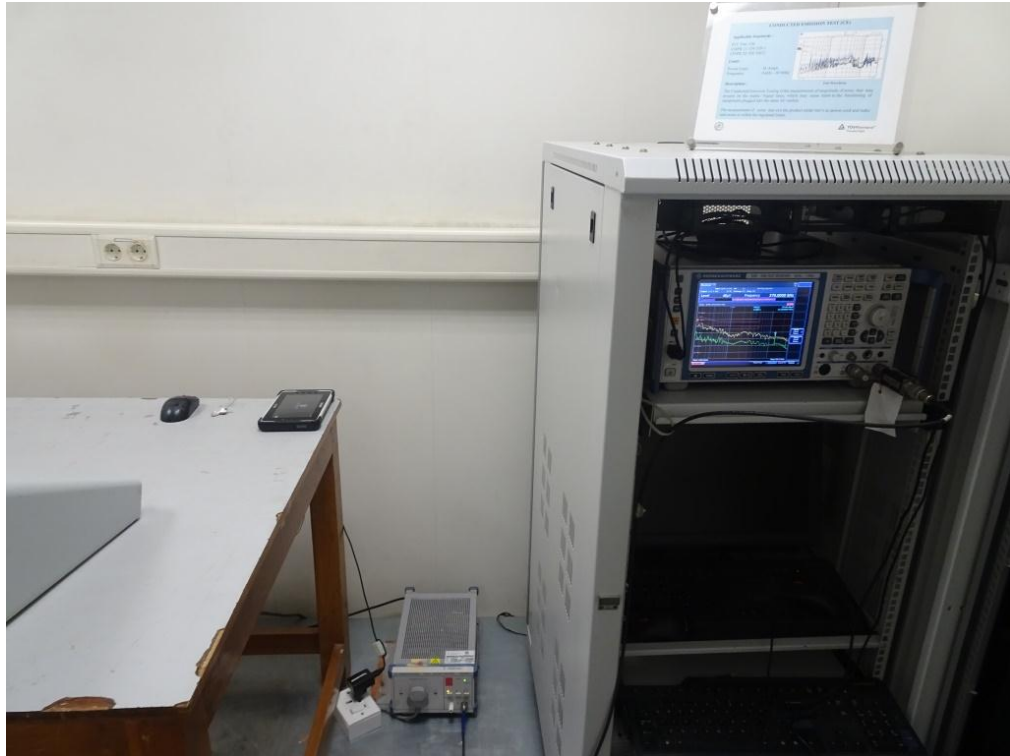
Conducted Emission Test setup
