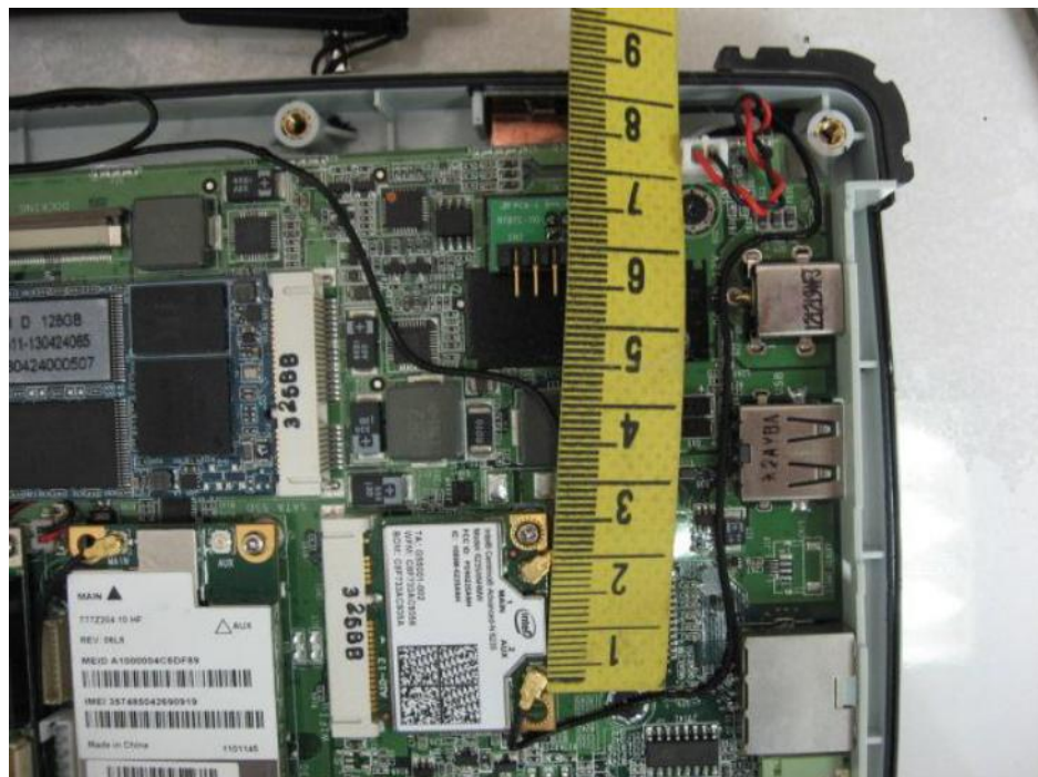
2G/3G Transmit Antenna
