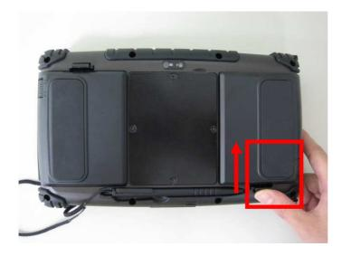
Step 2 Press up the compression lock from the tablet pc.
