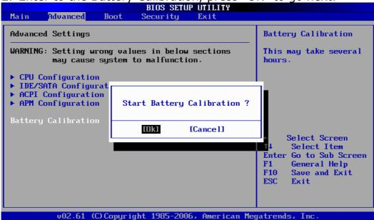
When you Push "OK" to start Battery Calibration, following below indicated to regulate the battery.
