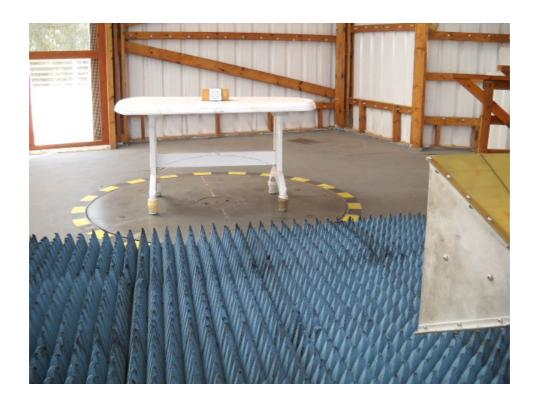
$\label{eq:Photograph No.6} Photograph \ No.6$  Setup for spurious emission field strength measurements at the OATS in 18 – 24.5 GHz
