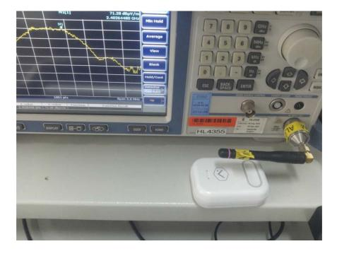
Photograph No.5 Setup for occupied bandwidth measurements
