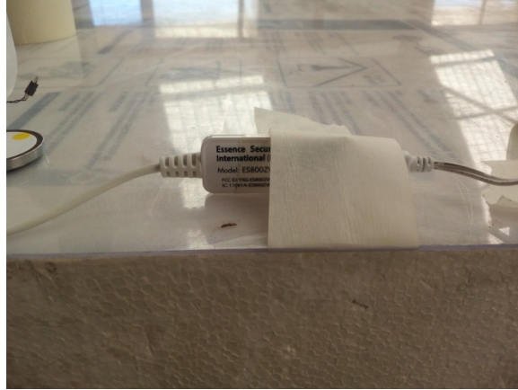
Photograph No.7 Setup for carrier emission measurements at the OATS, EUT in 3 orthogonal positions
