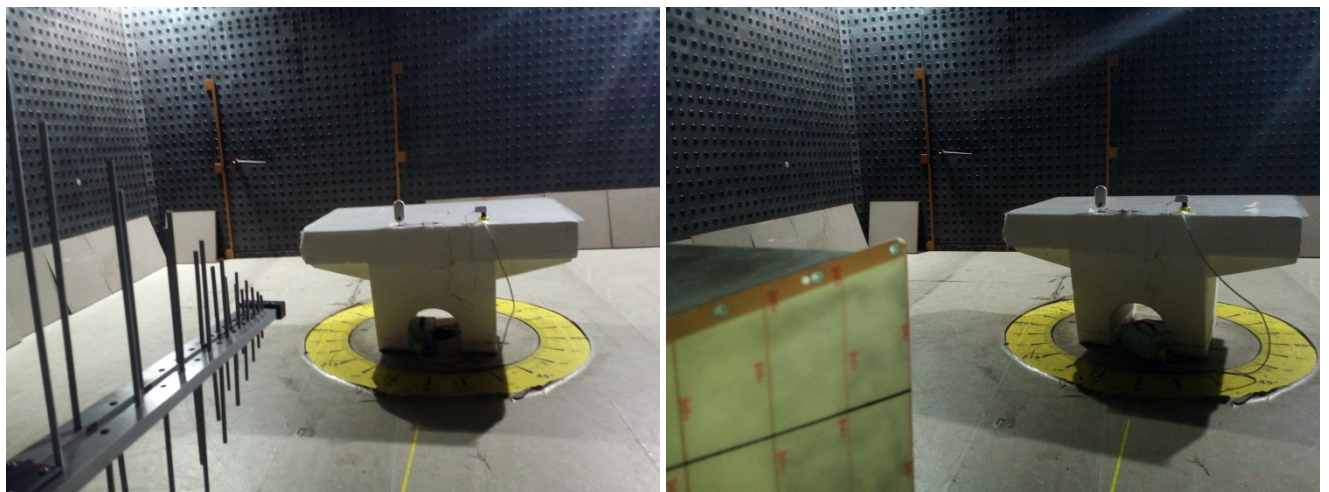
Photograph 8.2.1 Setup for radiated emission measurements in the anechoic chamber
