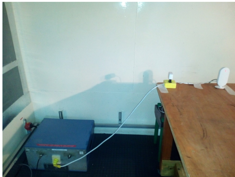
Photograph 8.1.1 Setup for conducted emission measurements
