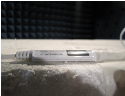
Photograph 6.6.3 EUT in Z-axis orthogonal position
