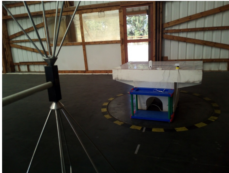
Photograph 8.2.3 Setup for radiated emission measurements, EUT cabling
