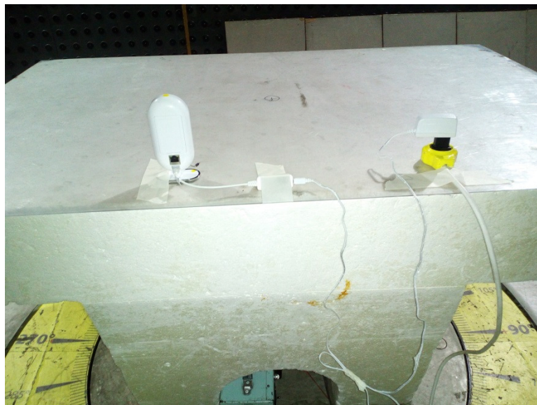
Photograph 8.2.3 Setup for radiated emission measurements, EUT cabling
