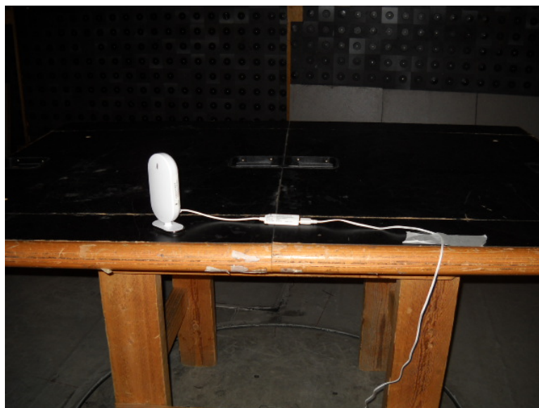
Photograph 8.2.2 Setup for final radiated emission measurements, EUT cabling
