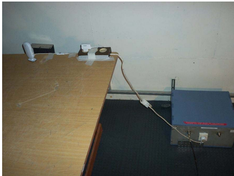
Photograph 8.1.1 Setup for conducted emission measurements
