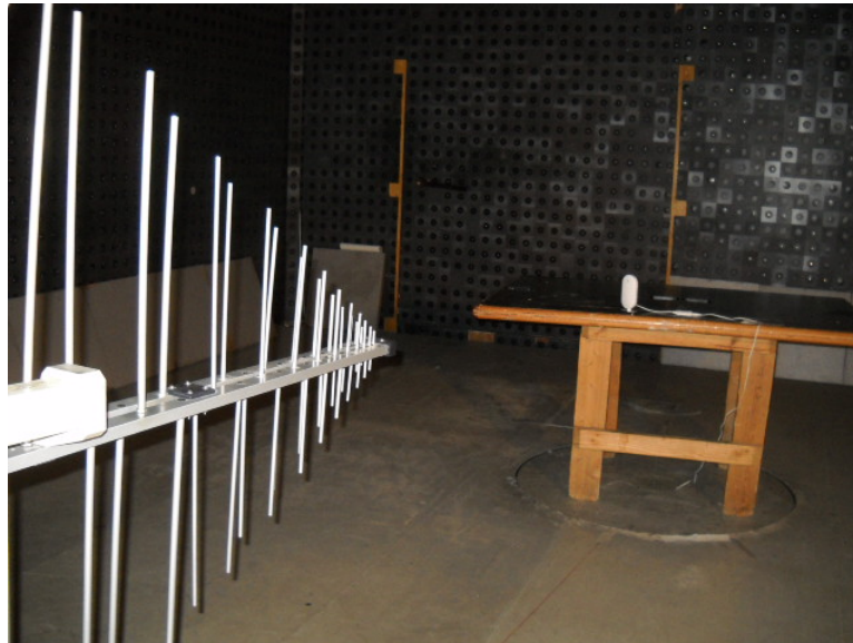
Photograph 8.2.1 Setup for radiated emission measurements
