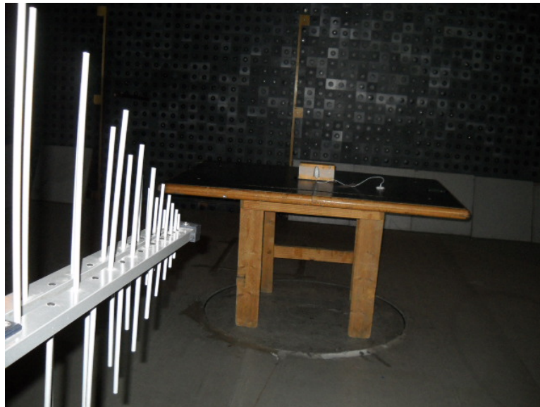
Photograph 8.1.1 Setup for radiated emission measurements
