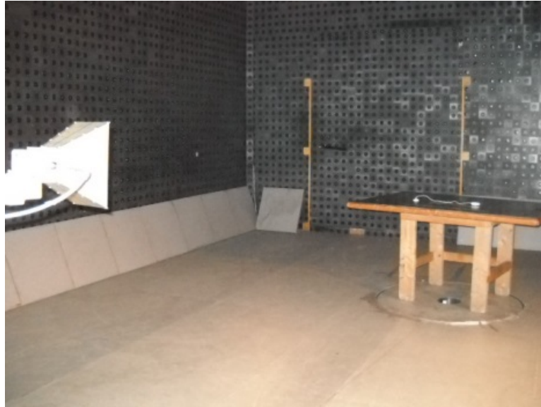
Photograph 8.1.2 Setup for radiated emission measurements
