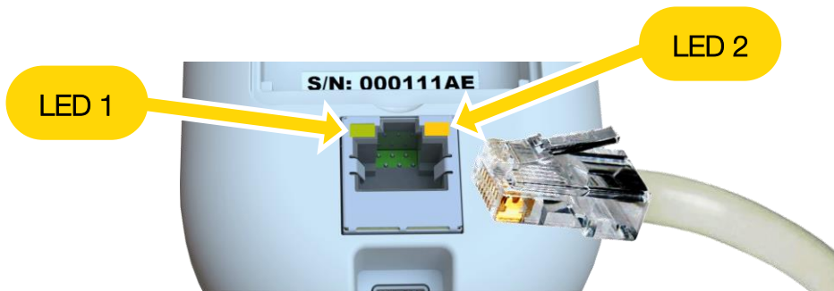
Figure 7: Insertion of LAN Cable into the CCU Socket
