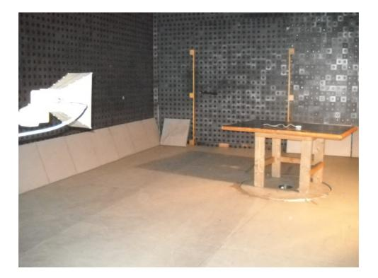
Photograph No.4 Setup for field strength measurements in the anechoic chamber, EUT close view
