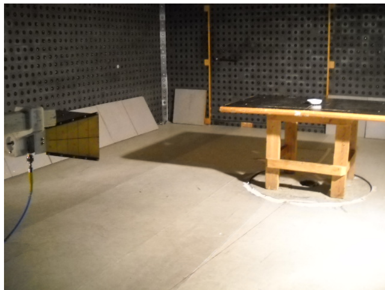
Photograph 7.2.1 Setup for carrier field strength measurements
