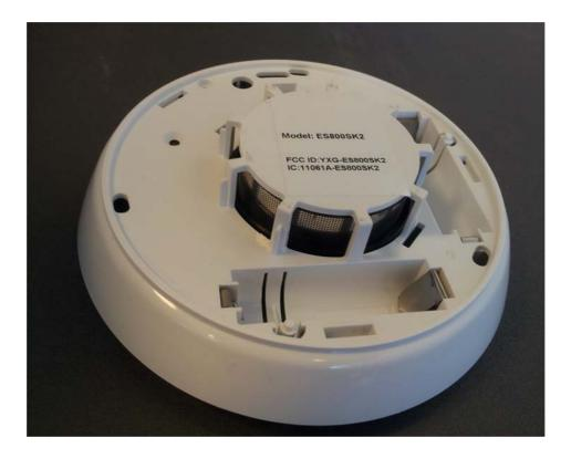
Label with FCC ID:YXG-ES800SK2 and IC:11061A-ES800SK2 is located at the rear side panel. The statement according to FCC part 15 §15.19(a)(3) is placed in User's Guide (Application exhibit User\_manual\_24461).
