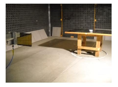
Photograph No.4 Setup for spurious emission field strength measurements at the OATS above 1 GHz
