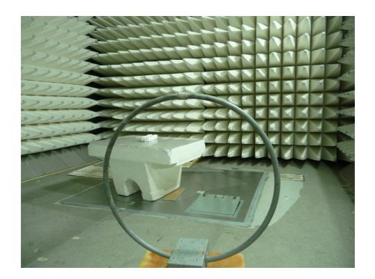
$\begin{array}{c} Photograph \ No.2 \\ Setup \ for \ carrier \ and \ spurious \ emission \ field \ strength \ measurements \ in \ the \ anechoic \ chamber \\ in \ 30-1000 \ MHz \ range \end{array}$
