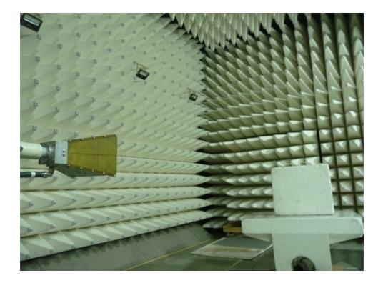
$\label{eq:Photograph No.4} Photograph No.4 \\ Setup for spurious emission field strength measurements in the anechoic chamber in 18 – 25 GHz$
