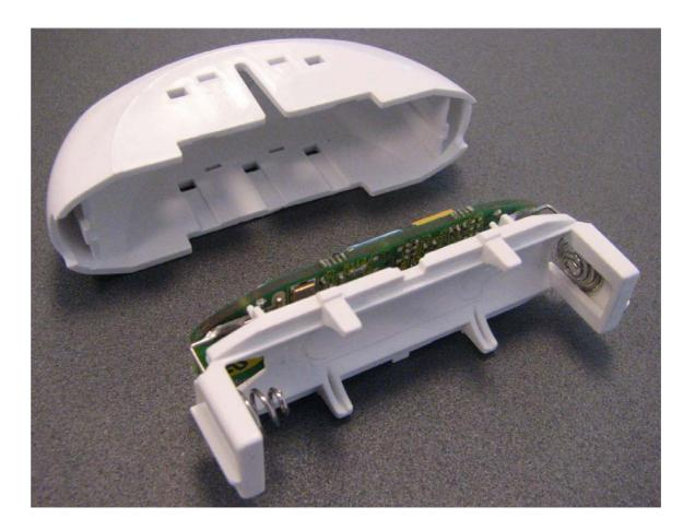
Photograph No.2 ES800MGL magnet sensor (detector) with case removed
