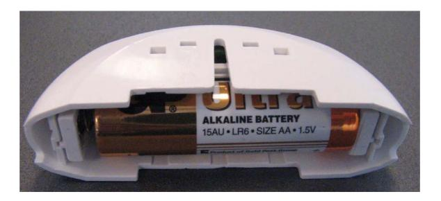
Photograph No.1 ES800MGL magnet sensor (detector) internal view with battery
