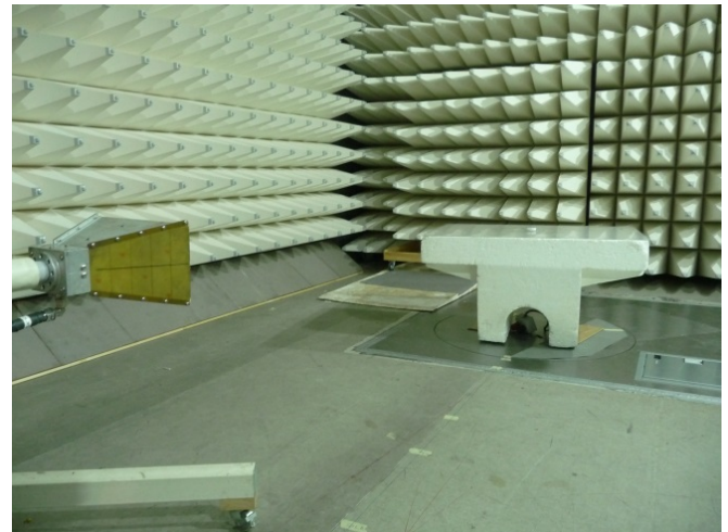
Photograph 8.1.1 Setup for radiated emission measurements
