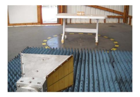
$\label{eq:Photograph No.6} Photograph No.6 Setup for spurious emission field strength measurements at the OATS in 18 – 24.5 GHz$
