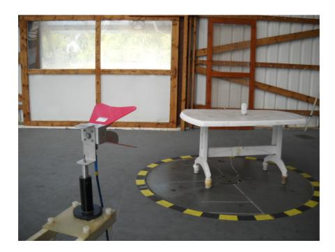
Photograph No.5 Setup for spurious emission field strength measurements at the OATS in 18 GHz – 25 GHz
