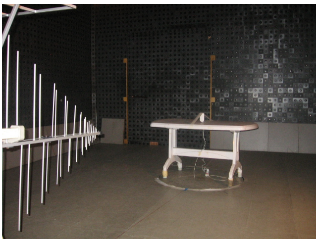
Photograph 8.2.1 Setup for radiated emission measurements
