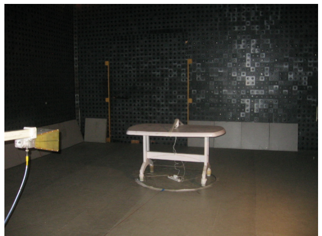
Photograph 8.2.1 Setup for radiated emission measurements
